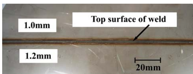
Fig. 3 Weld surface of TWB produced under optimal parameters
